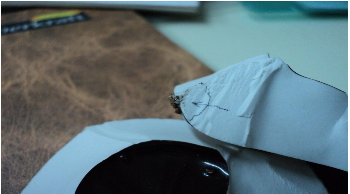
DISC INSULATOR FAILING UNDER THE TEST DUE TO GROG PENETRATION
