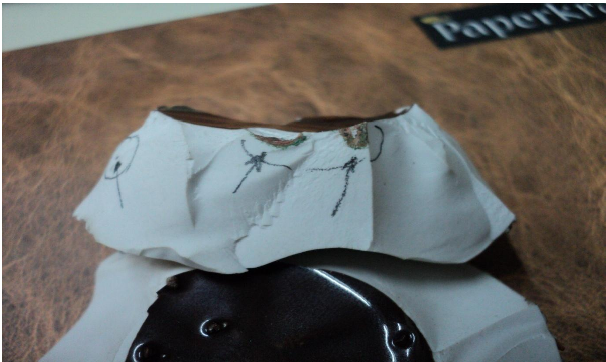
DISC INSULATOR FAILING THE TEST DUE TO MULTIPLE DEFECTS
